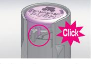
The plastic spring structure makes a clicking sound when the button is pressed.
