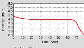
[Test condition] Saline solution is infused to CIA30-2040(4mL/h) at room temperature of 23°C
